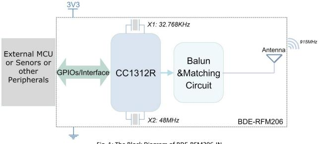
Fig. 1: The Block Diagram of BDE-RFM206-IN
