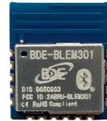
BDE-BLEM301 is compatible with Dialog DA14531 TINY™ Bluetooth Module - DA14531MOD. The same software tools and hardware kits can be used for BDE-BLEM301. It is empowered with Dialog BT5.1 qualified BLE stack and SDK with a rich set of software functions & examples to kickstart your development.
