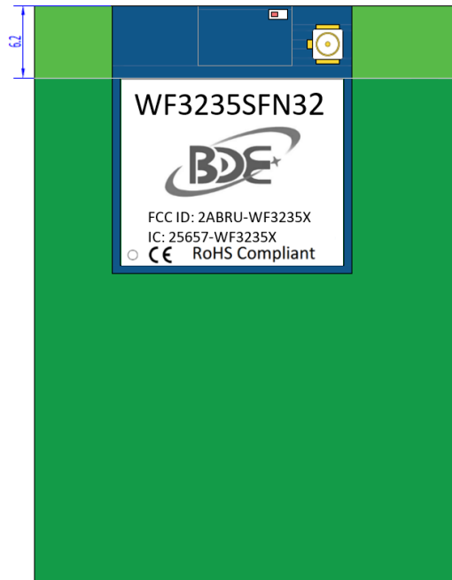
Figure 6-3. WF3235 Layout Guidelines
