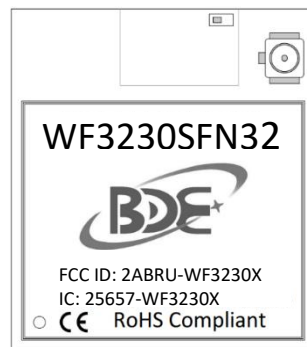
Figure 5-3: Indicative Module Shield Marking
