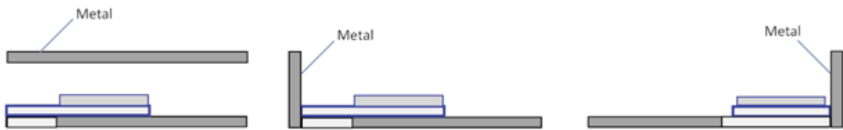
Figure 5-4. Not recommended location in Z plane
