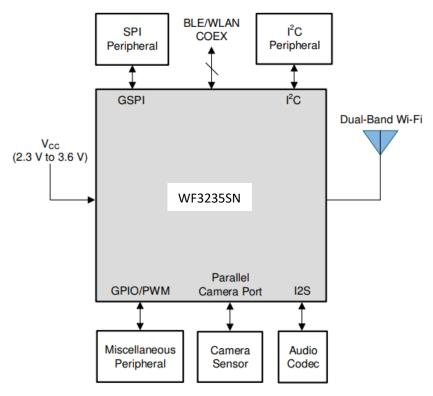
Figure 5-1. Functional Block Diagram
