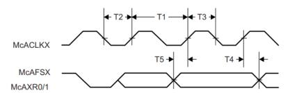
Figure 4-8. I2S Receive Mode Timing Diagram
