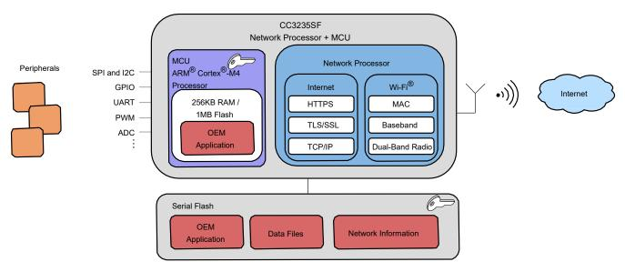
Figure 5-2. CC3235SF High-Level Structure
