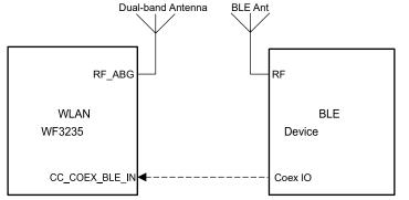
Figure 6-1. Dual-Antenna Coexistence Mode Block Diagram
