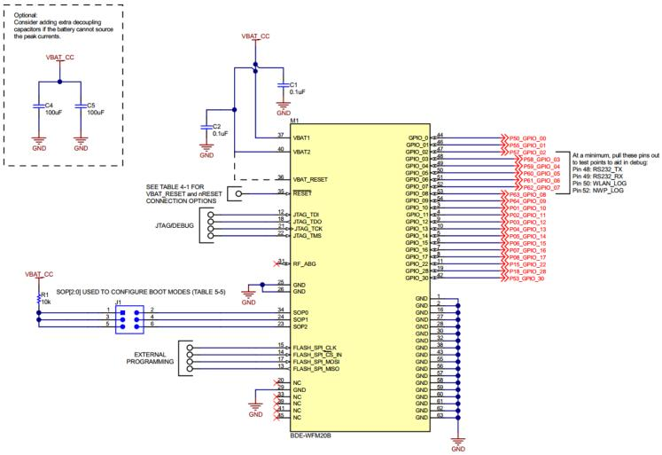
Figure 6-2. BDE-WF3235 Typical Application Schematic
