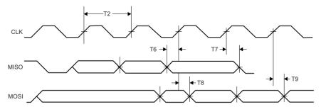
Figure 4-5. SPI Master Timing Diagram
