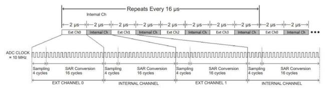
Figure 4-12. ADC Clock Timing Diagram
