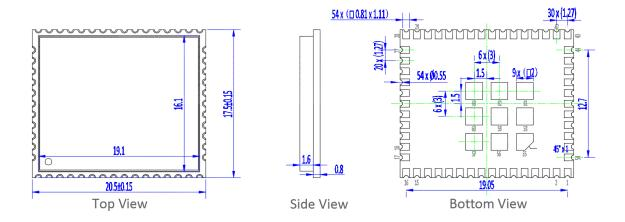
Figure 7-1: Mechanical Drawing
