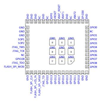
Figure 3-1. Pin Diagram Bottom View
