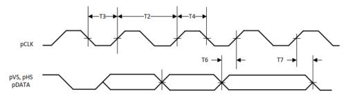
Figure 4-13. Camera Parallel Port Timing Diagram
