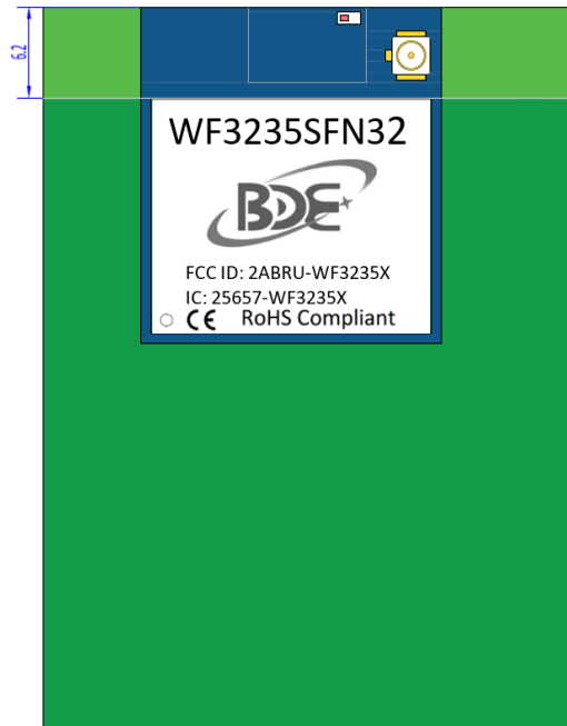
Figure 6-3. BDE-WF3235 Layout Guidelines
