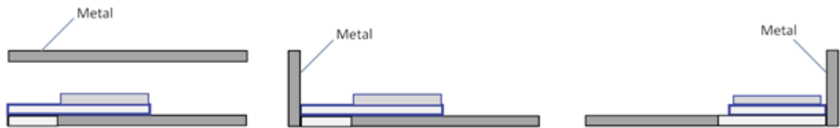
Fig 5-4. Not recommended location in Z plane
