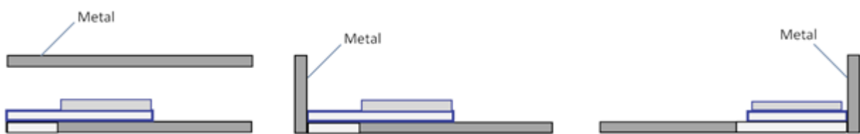
Fig 5-4. Not recommended location in Z plane
