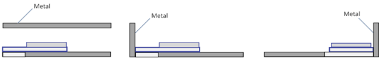
Figure 5-4. Not recommended location in Z plane
