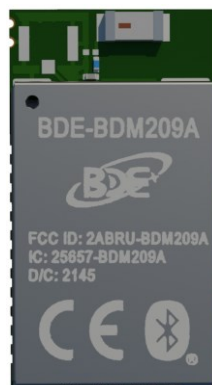
Figure 5: Indicative Module Shield Marking
