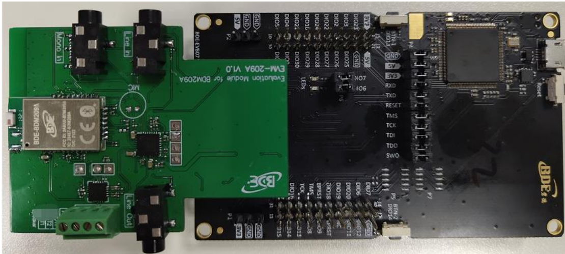
Figure 4-2: Plug BDE-EVM-209A in BDE-EVB07
